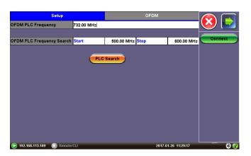
All OFDM measurements including the Subcarrier Power, MER, and Noise scans are available in this OFDM Check mode.
