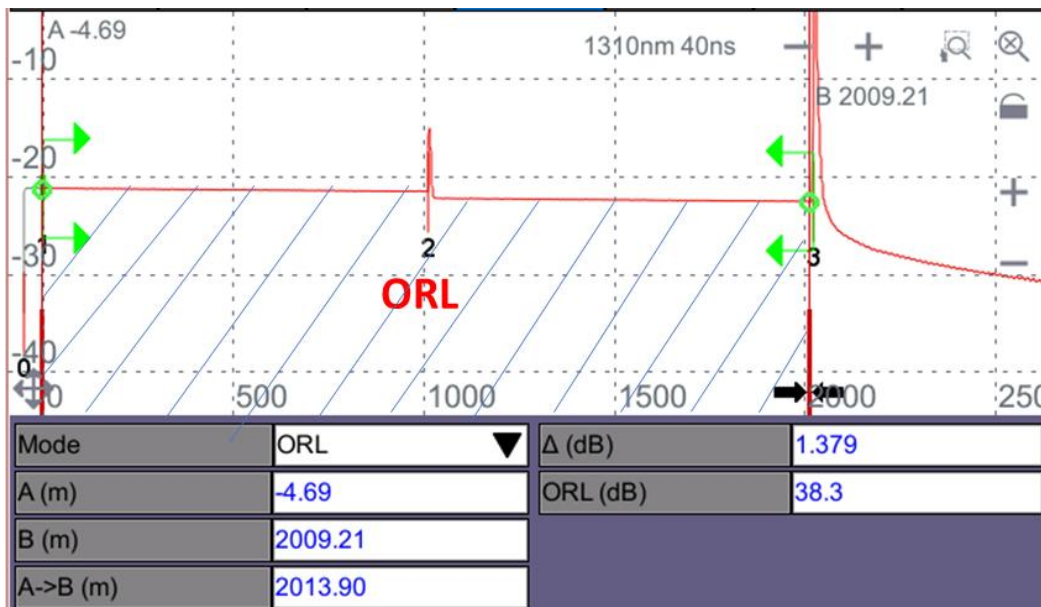
Figure 3: Trace graph showing an open end connector with high reflectance. This will result in erroneous failure of the ORL span if included in the link ORL measurement.
