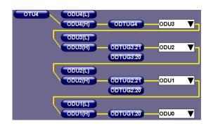
OTU4 multi-step mapping/multiplex structures
