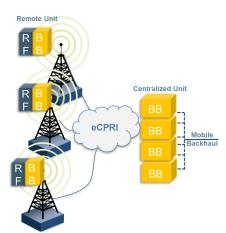
To ensure that 5G network's strict requirements are met in the fronthaul, the eCPRI Transport Network requirement document establishes classes of service for data and C&M traffic. With full line rate eCPRI traffic generation capabilities and high accuracy one-way latency measurements, the RXT6000e provides the tools necessary to ensure that the eCPRI transport network is ready for 5G deployments.
