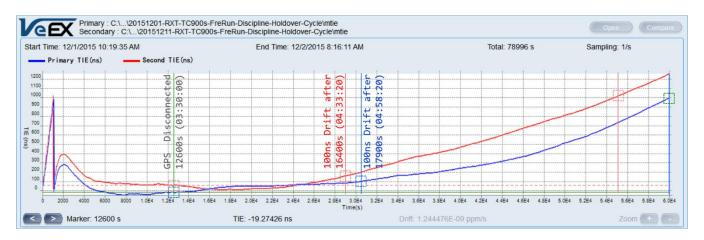
As expected, the two traces are slightly different. There is a baseline offset of about 70ns between the original and the new TE traces, which could be due to the internal GPS Clock plus the external GPS-disciplined reference uncertainties. Also, in the new test results (red) the first 100ns accumulate faster (25 minutes earlier) and reaches the 1,000ns mark earlier, after 42,000s of holdover.
