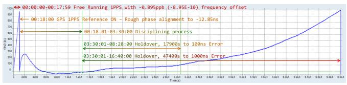
This graph depicts the full Time Error (TE) cycle of a test set's internal 1PPS reference, starting from free running, disciplining, to holdover. A relatively short holdover behavior was selected as an example, so all the different phases can be easily visualized.
