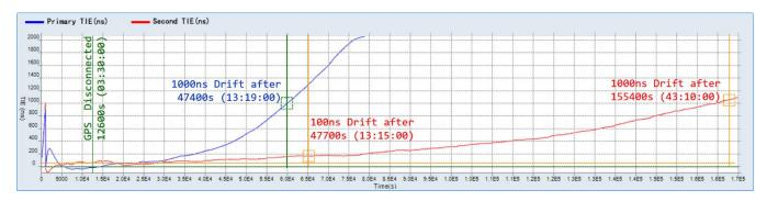
In this last example (red), the test set runs for more than 13 hours before accumulating 100ns error and it takes more than 43 hours to accumulate 1,000ns error. Significantly better than the original (blue) one, and it was also a
