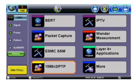
4. Configure the test set as a Slave and select whether it is a Layer 2 or Layer 3 UDP PTP environment.
