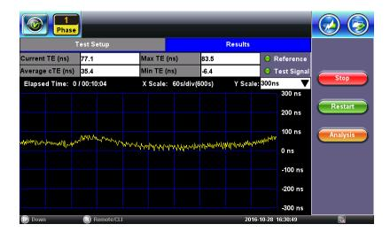
The TIE samples will always vary (wander) over time, but in a well-synchronized DUT it will slowly vary around Ons and it shall not diverge, neither in a positive nor negative direction. (A noisy DUT/SUT was selected on purpose for this example, for better illustrative purposes.)
