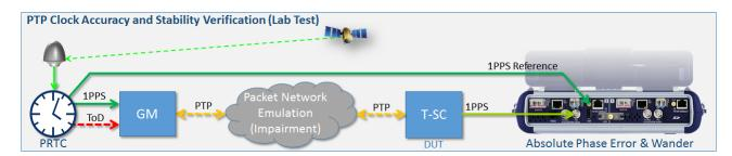
To measure the Wander or Phase Error at the Slave's physical clock output, use the Clock Wander Measurement test mode, which can be launched from >Additional Tests >Clock Wander & Phase Meas. In this case, you can connect the clock signal under test to RX1 (BNC) and the frequency or phase (1PPS) reference to the CLK (SMA) port or use the optional built-in precision timing and frequency references, if available.
