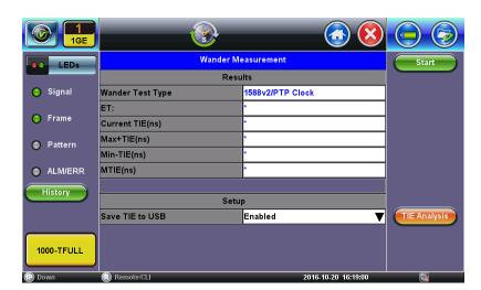
10. Press **Start**, enter the desired file name (no spaces) for the test result and press **Apply**. It is recommended to use meaningful file names, perhaps including the date for future reference (e.g. "ACME\_Bank-20161231")
