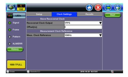
In this example, the test set is also configured to output a copy of its recovered clock on the TX1 (BNC) port.
