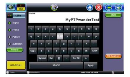
11. The Wander measurement starts and all the samples are saved in the USB memory for future analysis. The TIE from the recovered raw 1PPS clock will vary, but in a well-synchronized slave it will vary (wander) around Ons and not diverge in positive or negative direction. Of course, this all depends on the network under test.
