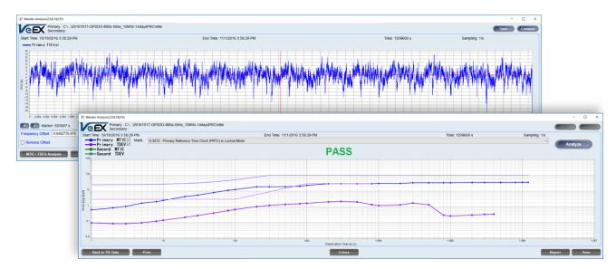
The 14-day TE example shows the long-term accuracy and stability of a TX320S test set with built-in GPS-disciplined Atomic Clock in locked condition and in a variable temperature environment. For this case TE =  $\pm 16$  ns, or Max|TE| = 16ns, and it passes the G.8272 PRTC MTIE and TDEV masks.
