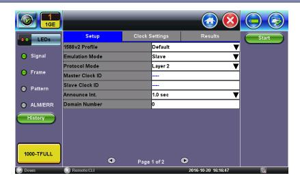
If Layer 3 is used, go to the IP function in the Main Menu to stablish and IP connection, before configuring the slave emulation. Then go back to configure the protocol Transfer Mode as Unicast or Multicast, and any other applicable settings to match the network.
