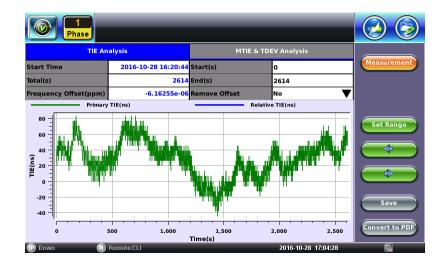
Users can also tap on the TIE graph to position a cursor, then use the  $\Leftrightarrow \Rightarrow$  arrow buttons to adjust the position to the desired sample.
