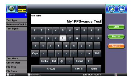
7. Press **Start**. The Wander measurement starts and all the samples are saved in real-time to the USB memory for future analysis. A 600-second monitoring graph shows the latest TIE or TE samples for users to evaluate the current status of the test and decide whether to continue, stop or abort the test (e.g. there is no point
