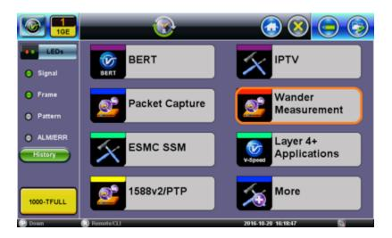
9. Insert a FAT32 USB memory stick in a USB port, wait until the 🌶 icon appears on the top-right corner of the screen and Enable the Save TIE to USB. The sampling rate may be limited to one TIE measurement per second.
