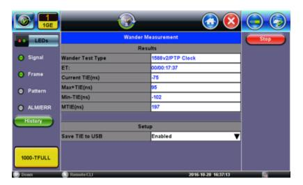
If you need to check the up-to-the-moment TIE results while the test is still running, you can use the Open Files procedure described later on in the "Built-in Post Analysis" section.
